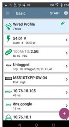
NBASE-T network with VLAN and 802.1x authentication
